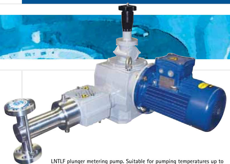
LNTLF plunger metering pump. Suitable for pumping temperatures up to 280°C thanks to cooling jacket and special materials of plunger packing.
