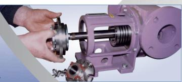
To easily dismount the mechanical seal from backside, a ball bearing cartridge is available on request.
